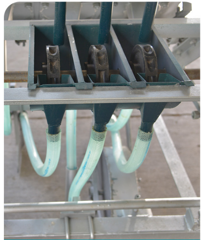
Fertilizer metering chute
